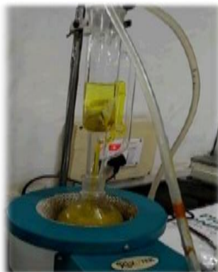
Fig.2: Extraction of Curcumin from rhizomes of turmeric
