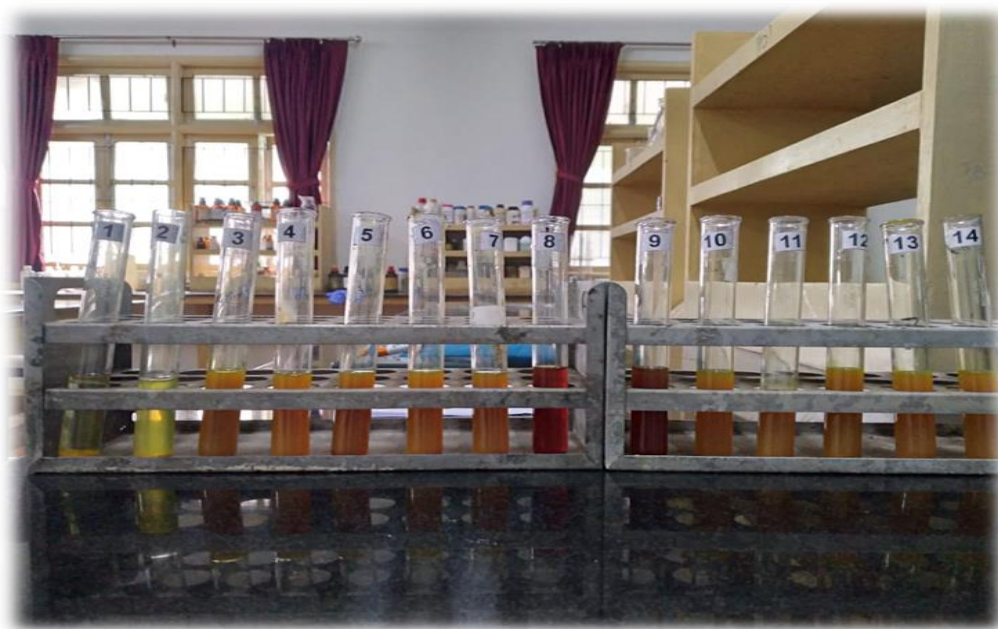
Fig.8: Color change in different pH solutions
